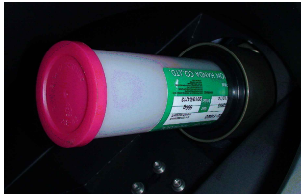
Insert the barrel Type solder bottle
